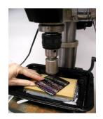
Before you begin coring you will need to get some idea of WHERE you want to make your first cut. While holding the glass firmly against the wood block, you will gently lower the pilot feed lever until the drill bit makes contact with the
